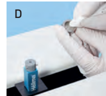
Clean window and cap (TrayCell remains in spectrophotometer).
