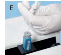
Pipette new sample onto window.
