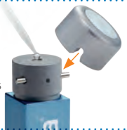
Remove cap and recover sample if necessary.
